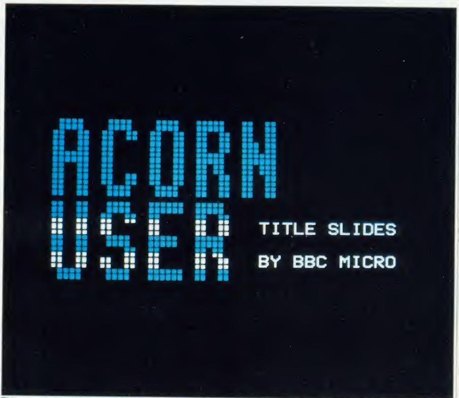
This simple title slide was quickly created with Beebugsoft's Teletext Pack teletext editor in mode 7
